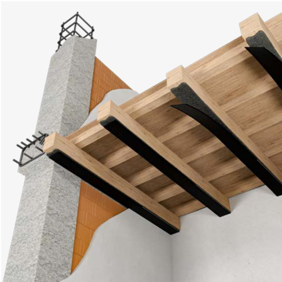
Illustrative rendering - intervention with laminates on timber floor slab
