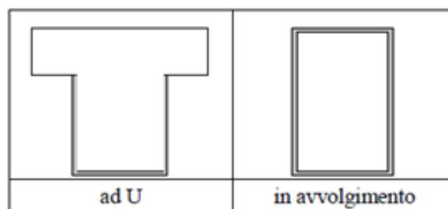
Fig. 23 - Shear reinforcement arrangement around the section.
