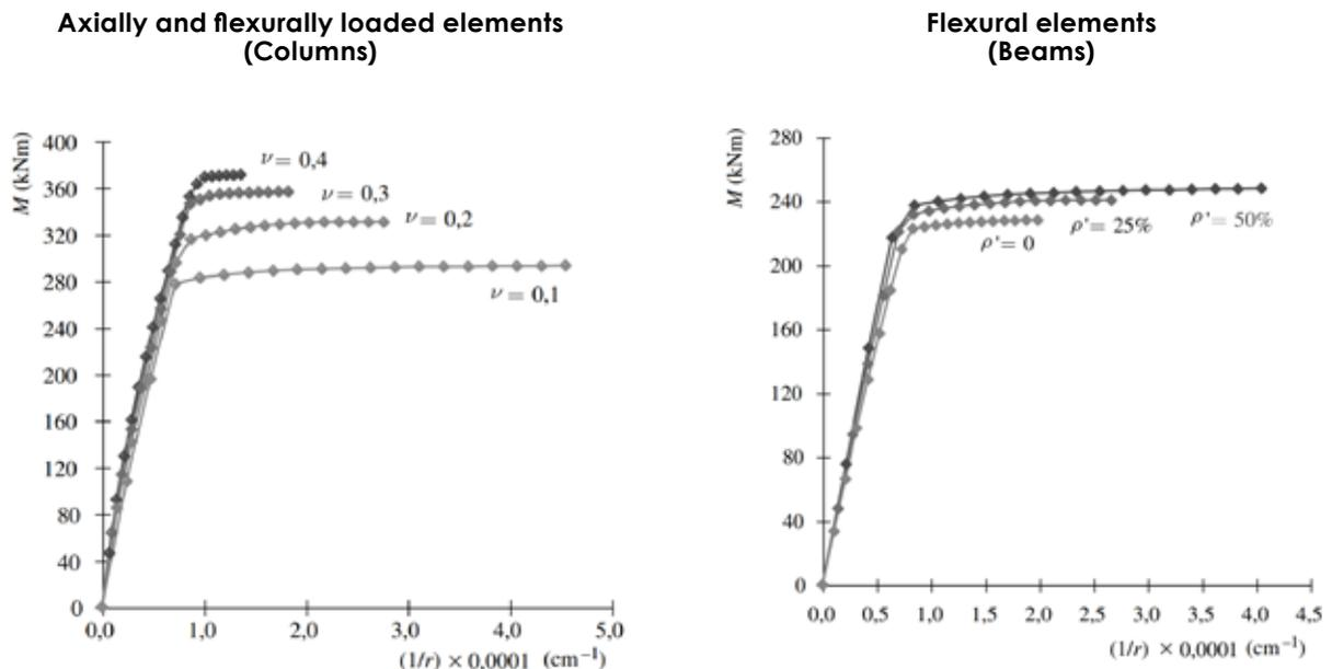
Fig. 12 - Moment-curvature diagrams for axially loaded (columns) and flexural (beams) sections [1]
