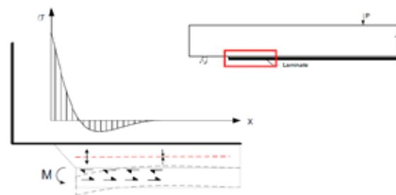
Fig. 05 - Peeling-induced debonding
