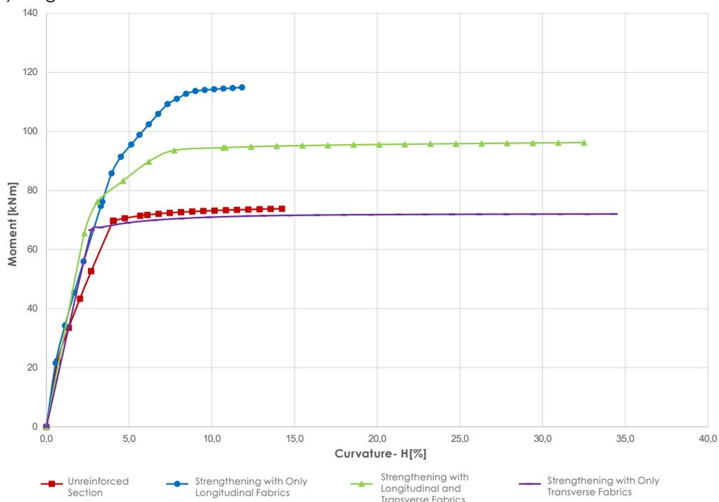
Fig. 21 - Comparison of moment-curvature diagrams: as-built state vs. different design scenarios
