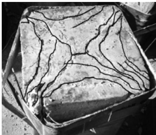
*Fig. 10 - Concrete element confined with carbon fiber fabrics*
