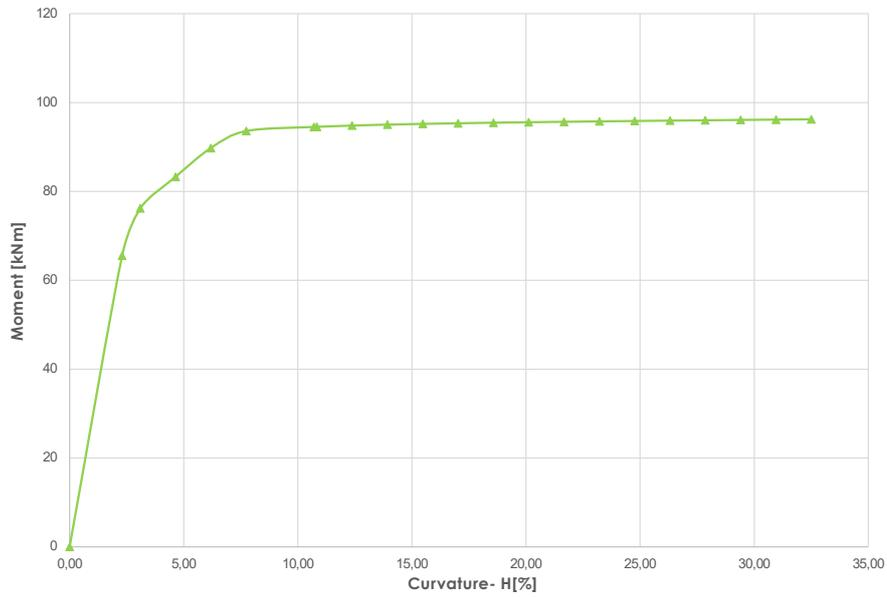
Fig. 19 - Moment-curvature diagram of the strengthened section (Hp. 2)
