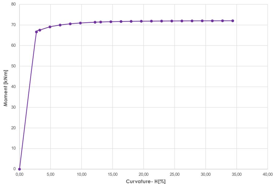
Fig. 20 - Moment-curvature diagram of the section at the design state (Hp. 3)
