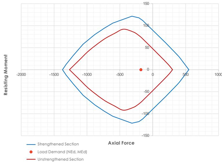
Fig. 15 - M–N interaction diagram of the strengthened reinforced concrete section
