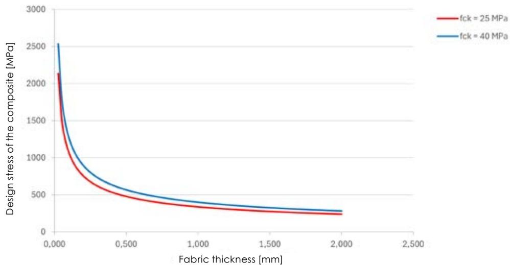
**Fig. 07** - Variation in bond strength with reinforcement thickness  $t_f$
