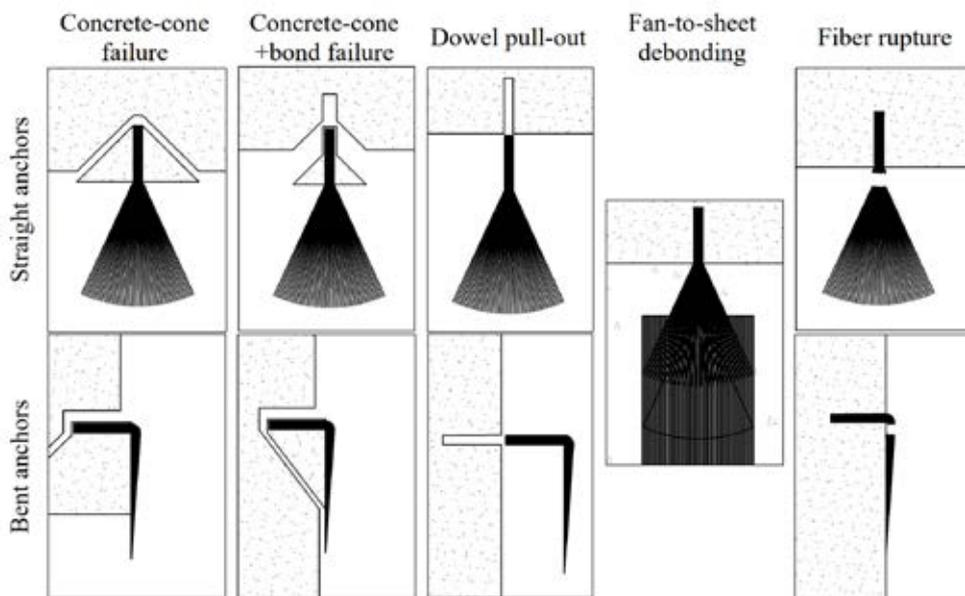
Fig. 28 - Failure modes of the connector
