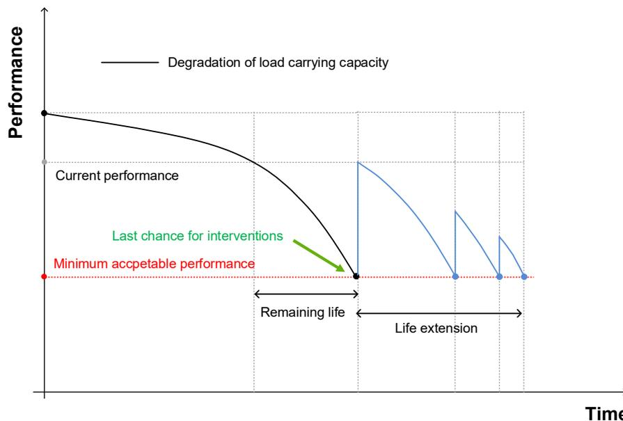
Fig. 01 - Extension of the service life of the structure following maintenance interventions (e.g., structural strengthening)
