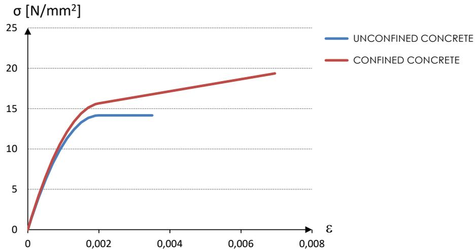
Fig. 11 - A typical stress-strain ( $\sigma$ - $\epsilon$ ) relationship of an FRP-confined concrete element
