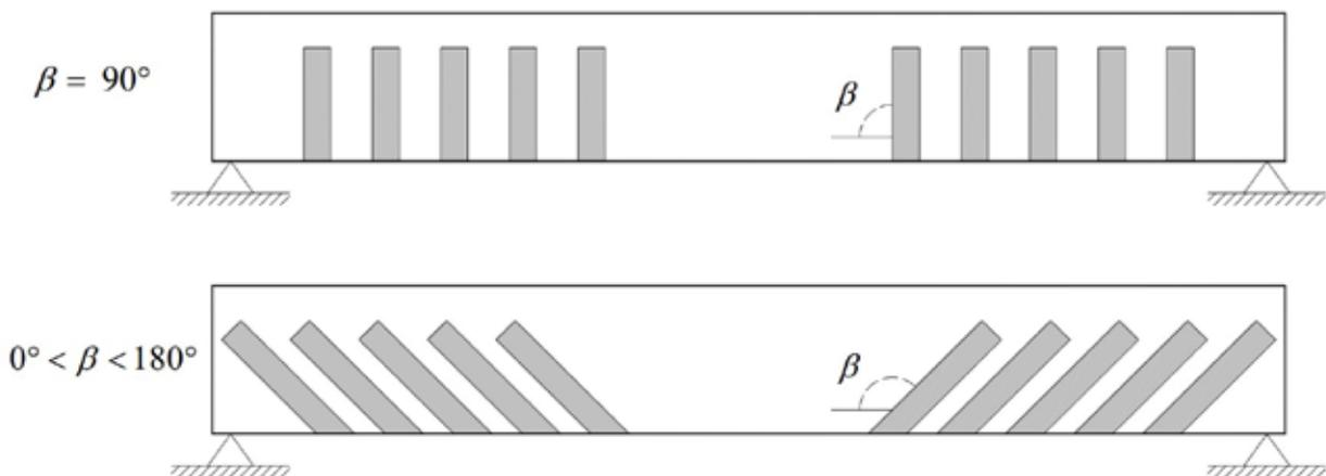
Fig. 22 - Shear reinforcement orientations using strip layout.
