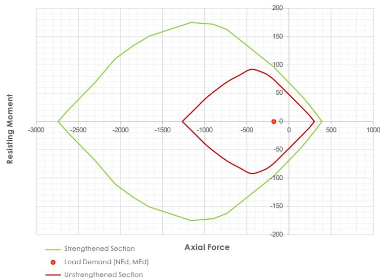
Fig. 18 - M–N interaction diagram of the strengthened reinforced concrete section
