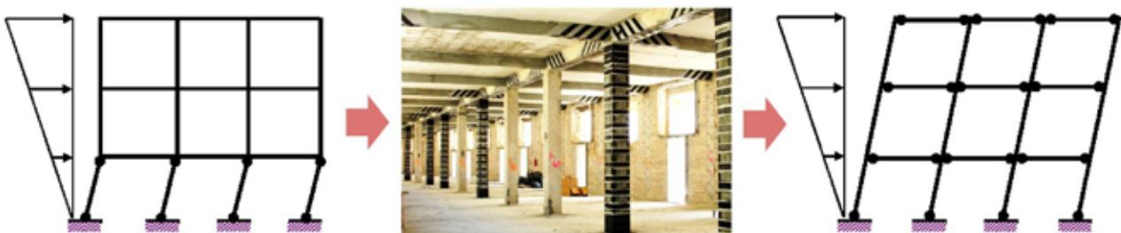
Fig. 02 - Composite materials can be used to modify the structural failure mode
