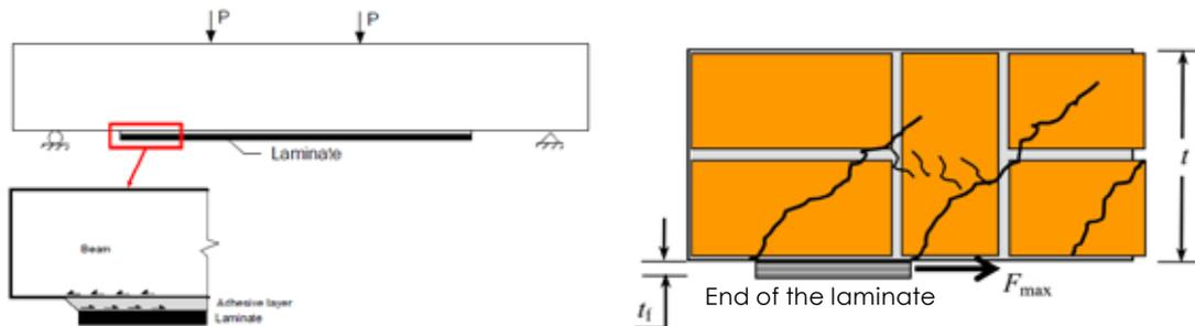
Fig. 03 - Debonding modes of composite reinforcement from concrete substrate
