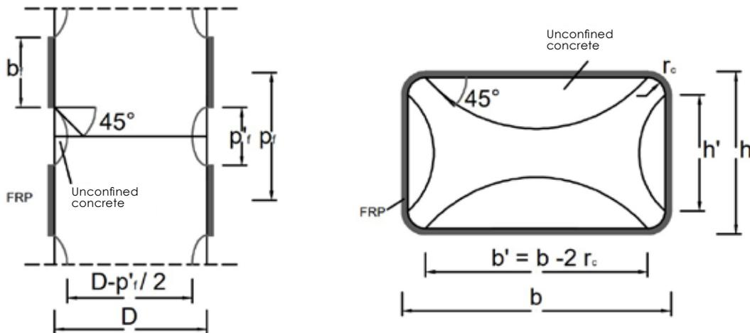
Fig. 17 - Confinement intervention on a reinforced concrete section using FRP reinforcements
