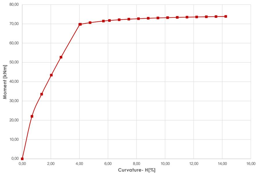
Fig. 14 - Moment–curvature diagram of the existing section.
