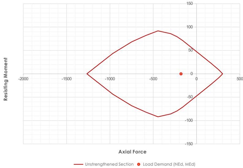
Fig. 13 - M–N interaction diagram of the existing reinforced concrete section
