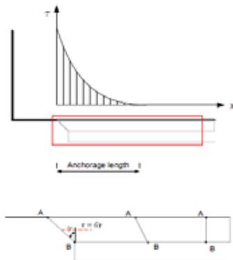
Fig. 04 - Debonding due to the development of maximum shear strength
