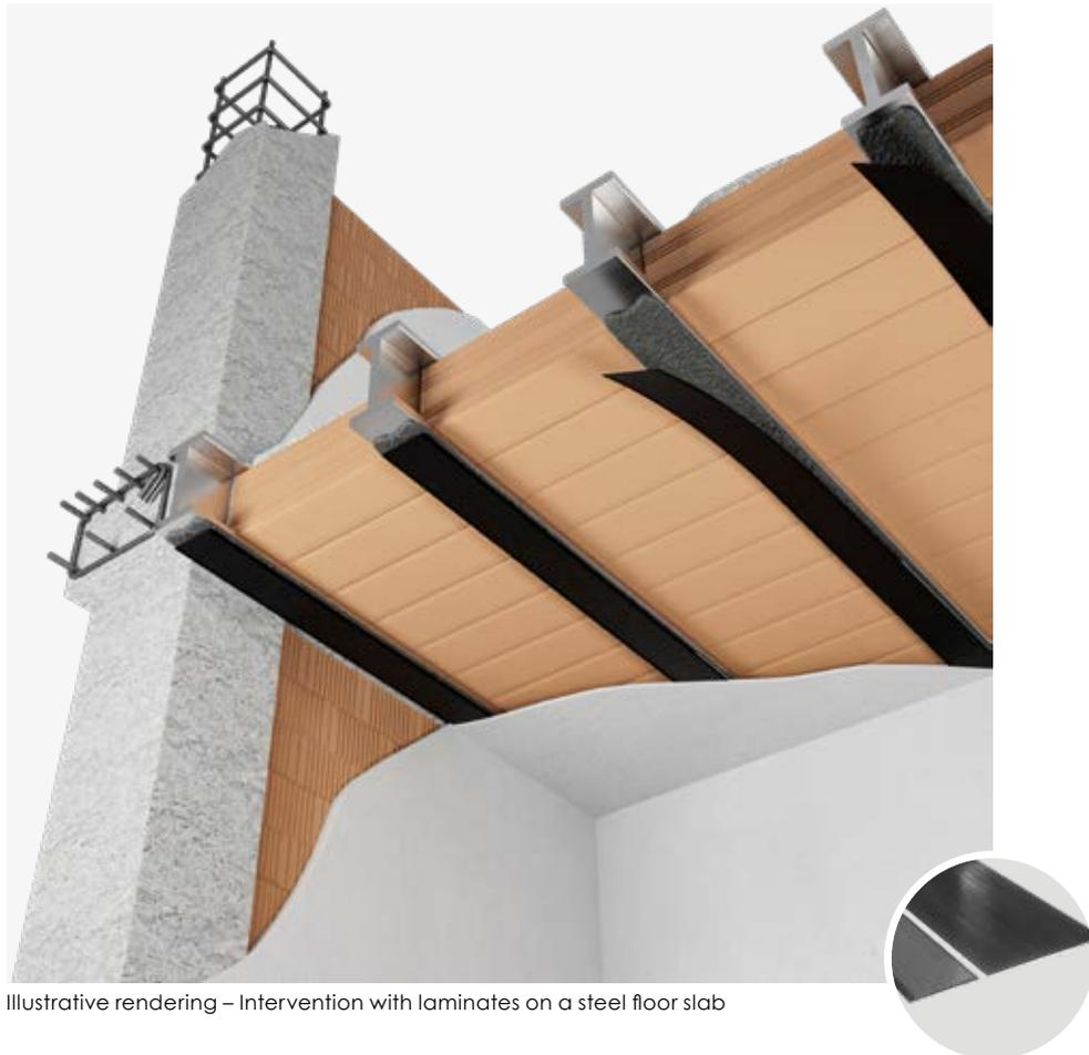
Illustrative rendering – Intervention with laminates on a steel floor slab
